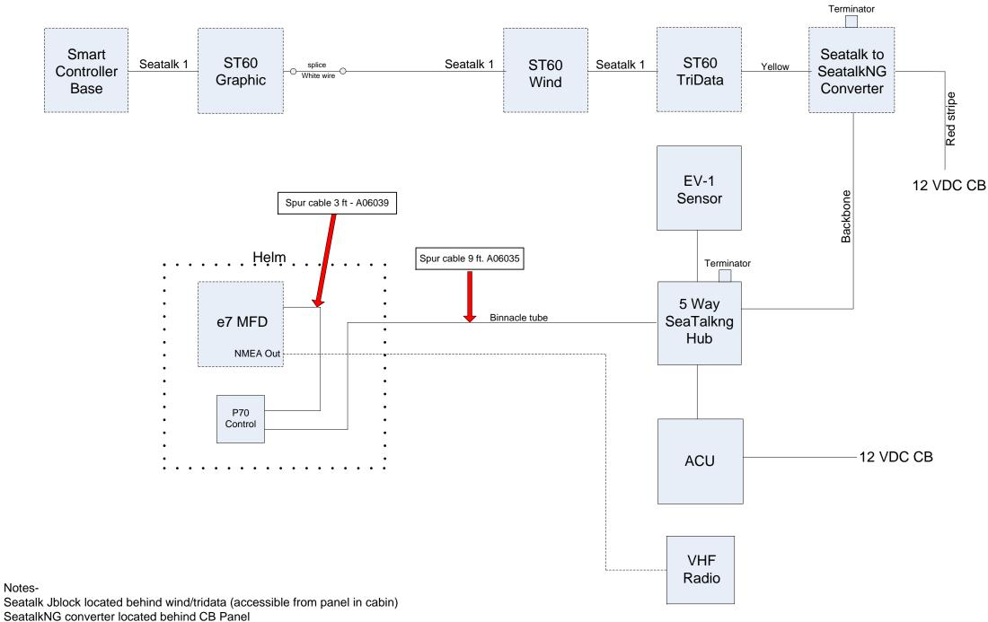
Smart Pilot Controller Base located on top of Engine Panel rear cover shell
