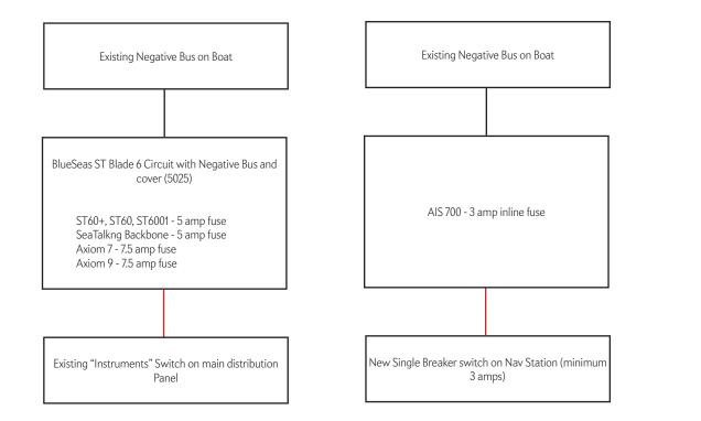
NEED TO UPGRADE INSTRUMENTS SWITCH TO at least 25 AMP IT IS CURRENTLY 10 AMP (also increase gauge of wire supplying this breaker switch to accomodate increased amps) Wire Gauges (Estimated lengths round trip)
