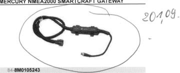
The Mercury NMEA2000 SmartCraft Gateway converts Mercury engine and system data to NMEA 2000 for use on non-Mercury gauges and displays for 1 to 4 engines. It also converts applicable NMEA2000 data to SmartCraft data for display by applicable SmartCraft gauges and displays. Includes a NMEA 2000 "T" connector for quick installation.
