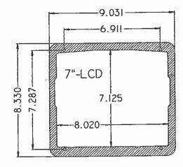
The sole purpose of this laser cut template is to simplify the installation of the Raytheon 7" and 10" monitor screens.
