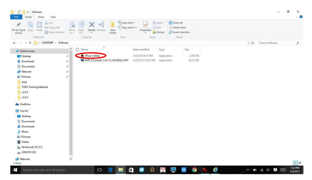
Determine the IP camera's IP address – Step 3: Left click on the <u>Scan</u> button within the IPScan Utility to initiate scanning for the camera's IP address.
