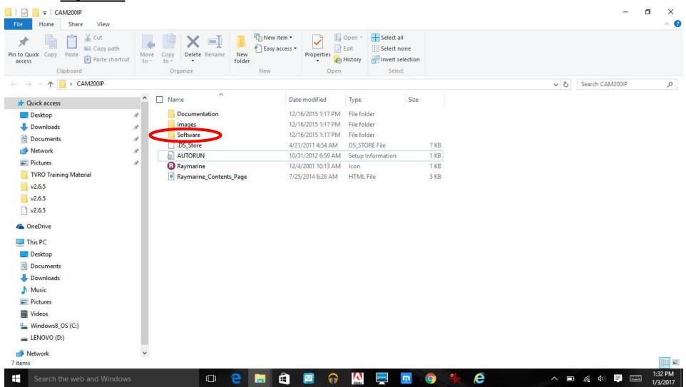
Determine the IP camera's IP address – Step 2: Double left click on the <u>IPScan Utility</u> executable file within the Software folder.
