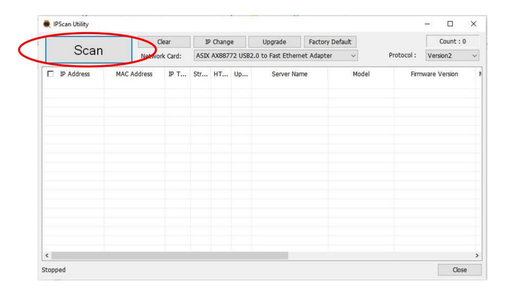
Determine the IP camera's IP address – Step 4: Note the IP Address (in this case 10.21.0.100) reported by the IPScan Utility for the IP camera which has been interfaced to the PC. Note that the IPScan Utility may additionally be used to determine the version of firmware installed within the IP camera.
