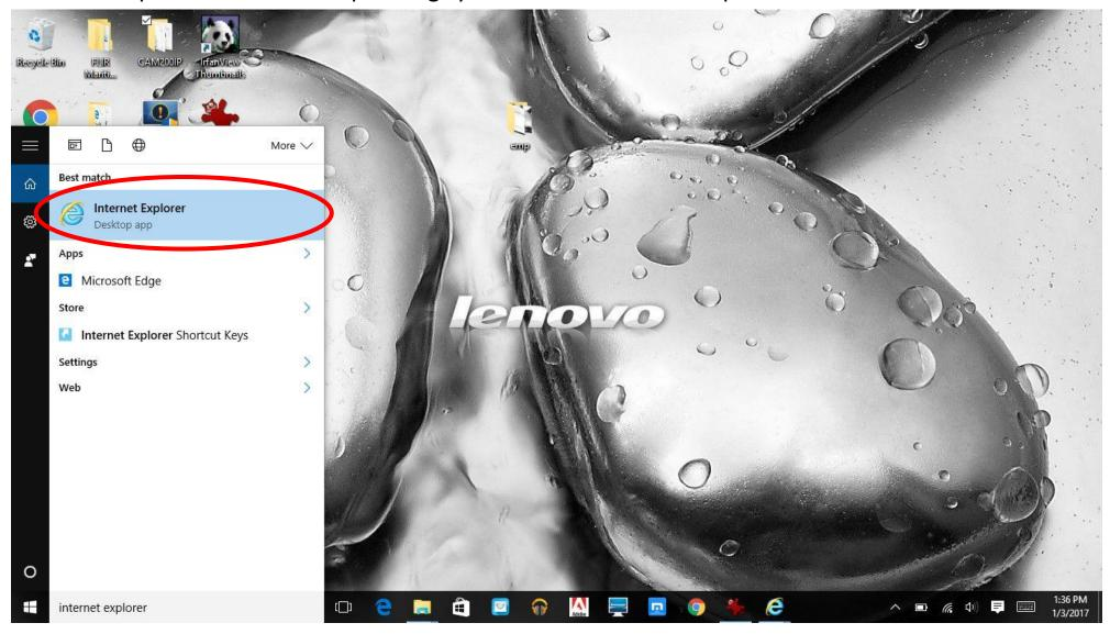
Open the IP Camera's web page – Step 1: Type the IP Camera's IP address into the address field of Internet Explorer and then press the **ENTER** button on the PC's keyboard.
