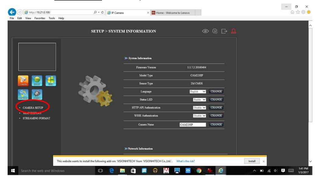
View/configure camera settings – Step 5: Changes to any of the setup parameters listed within the Camera Setup screen are instantly (i.e. do not require use of a save or apply button ... simply close the Internet Explorer window/tab when the desired changes have been made).
