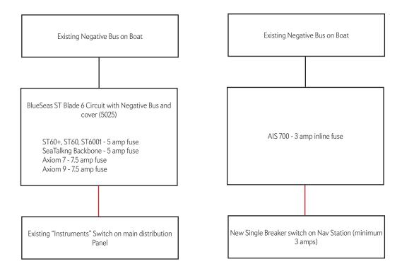
NEED TO UPGRADE INSTRUMENTS SWITCH TO at least 25 AMP IT IS CURRENTLY 10 AMP (also increase gauge of wire supplying this breaker switch to accomodate increased amps)
