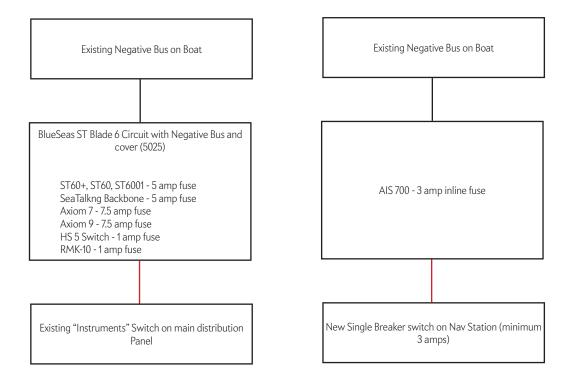
NEED TO UPGRADE INSTRUMENTS SWITCH TO at least 30 AMP IT IS CURRENTLY 10 AMP (also increase gauge of wire supplying this breaker switch to accomodate increased amps)
