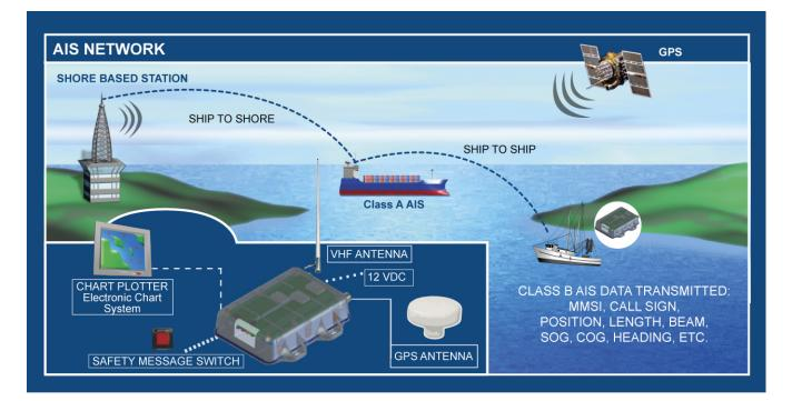
On the bottom, a typical NAUTICAST-B installation in a common environment is shown. The NAUTICAST-B is connected to the vessels power supply, and in connection with the VHF, and GPS-Antennas, the minimal requirements for Transponder operation are fulfilled.
