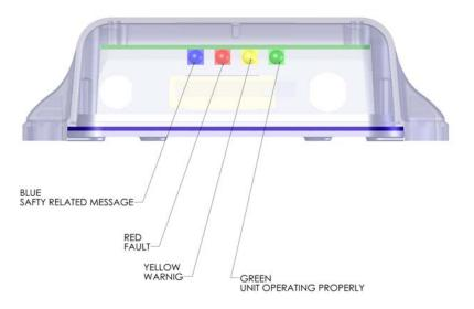
If the Red LED illuminates continuously the unit should be assumed to be faulty and should either be switched off (power removed) or if this is not practical any other vessel position information derived from the unit should not be used and it should also be assumed that the unit is not transmitting valid position information for your vessel.
