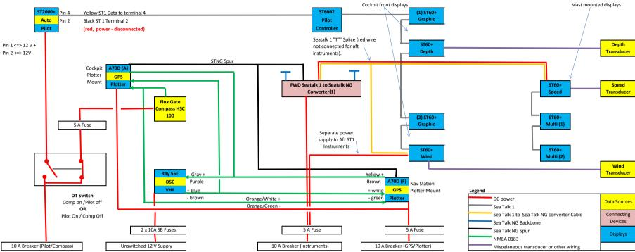
Notes 1. A70D has two mounting locations/plugs/STNG Spurs (cannot be present at both terminals)
