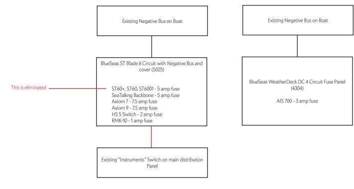
NEED TO UPGRADE INSTRUMENTS SWITCH TO at least 30 AMP IT IS CURRENTLY 10 AMP (also increase gauge of wire supplying this breaker switch to accomodate increased amps)
